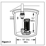
Flexible discharge NOTICE hose is intended for temporary use only. Rigid PVC or metal pipe is required for a permanent
